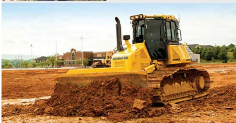
Baker's Construction & Excavation uses a Komatsu intelligent Machine Control D61PXi-23. "We love the D61i's integrated machine control," said Vice President Jeremy Baker. "The operator is always pushing the right amount of material, and it helps prevent overcutting, so we don't have to unnecessarily place and compact expensive replacement fill."
